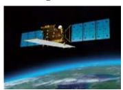
The state-of-the-art L-band Synthetic Aperture Radar-2 (PALSAR-2) aboard ALOS-2, which is active microwave radar using the 1.2GHz frequency range, will, in responding to society's needs, have enhanced performance compared to the DAICHI/PALSAR. The PALSAR-2 can observe day and night around the clock.
